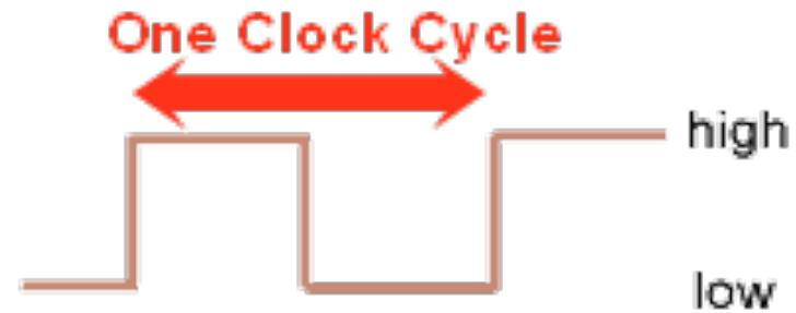
The digital signal from the clock controls the rate that the CPU executes instructions
